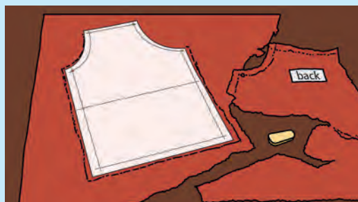
Figure 7.10: Uneven marking and cutting of fabric
